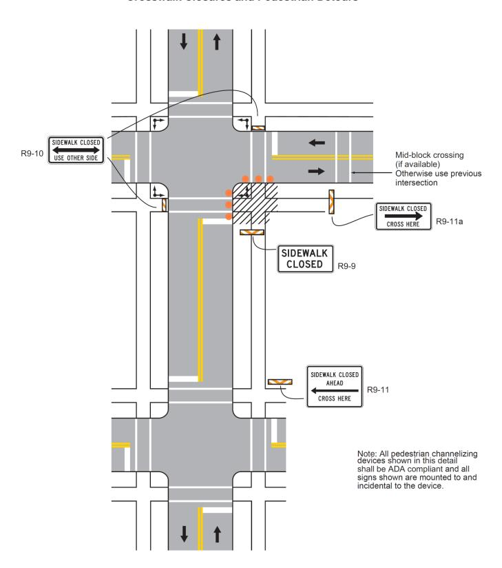
2022CPT.10.12.10901, 2022CPT.10.12.20901 **ADA COMPLIANT PEDESTRIAN TRAFFIC CONTROL DEVICES:**(10/31/2017)
